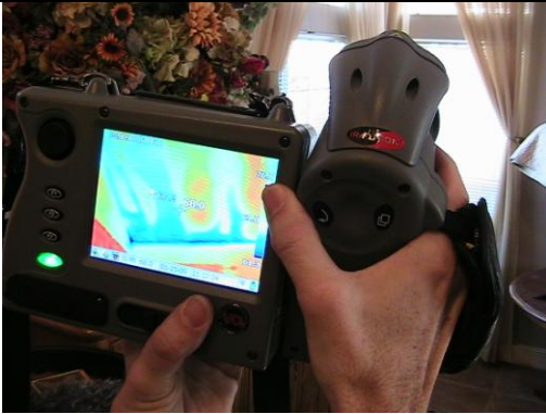
IR camera can see hot/cold spots in walls
